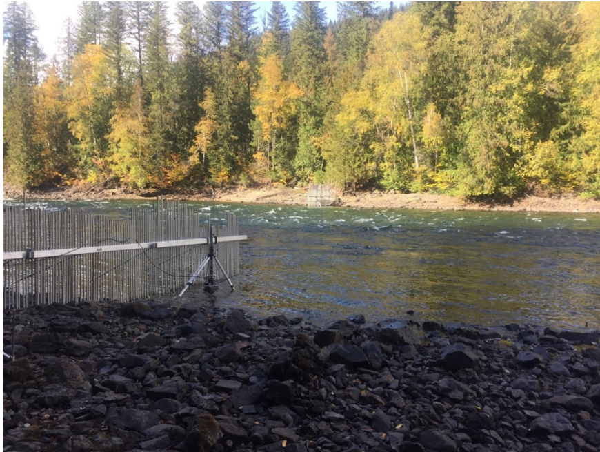
Figure 4. Left bank DIDSON and Right bank ARIS setup.
